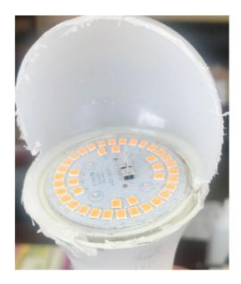
70. The heat sink of the A21 Series is capable of drawing heat from the LED devices, in particular, by drawing heat into the interior volume of the light source enclosure.
