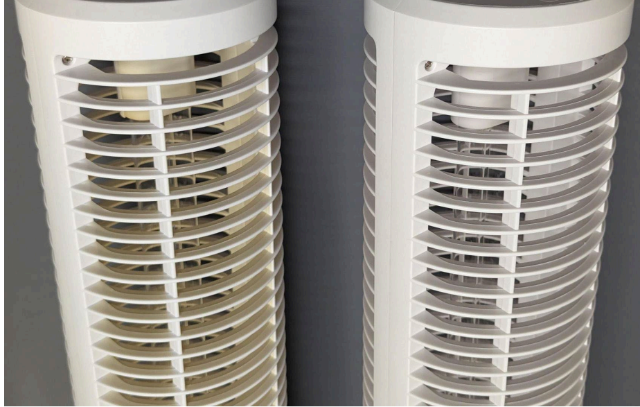
Figure 29. LPM-22-02C after three days of gonio testing (left) and unused LPM-22-02B (right).
