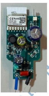
258. On information and belief, 901003-US-a products include a first antenna connected to the RF communication circuit for communicating RF control signals and arranged within the outer enclosure; for example, 901003-US products include an antenna connected to the RF module for communicating RF control signals—via the Wi-Fi protocol. The antenna is arranged within the plastic bulb of the lighting device, which comprises a portion of the outer enclosure.
