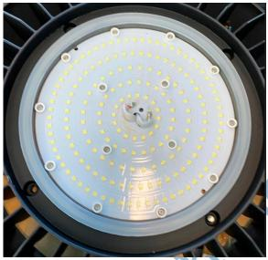
On information and belief, 3500013-DW-US products include a heat dissipation 114. element thermally coupled to the thermally conductive substrate; for example, 3500013-DW-US products include a heat dissipation element formed by a solid-metal body that includes a set of fins, which is thermally coupled to the metal-core printed circuit board.
