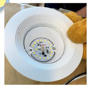
222. On information and belief, 170001-DW-US products include a driver electrically coupled to the at least one LED; for example, 170001-DW-US products include a driver electrically coupled to the LED light sources.
