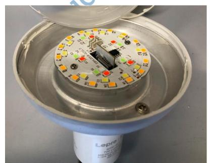
263. On information and belief, 907001-US products include a RF communication circuit; for example, 907001-US products include an RF communication circuit formed by a CB2L chip, a low-power embedded Wi-Fi module.
