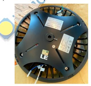
115. On information and belief, 3500013-DW-US products include a housing element including fastening means for detachably coupling the housing element to the heat dissipation element; for example, 3500013-DW-US products include a housing element, formed by a frame and transparent window. The housing element further includes screws, which pass through holes in the
