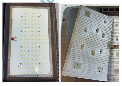
120. On information and belief, 620001-NW-US-LC products include a heat dissipation element thermally coupled to the thermally conductive substrate; for example, 620001-NW-US-LC products include a heat dissipation element formed by a solid-metal body that includes a set of fins, which is thermally coupled to the metal-core printed circuit board.
