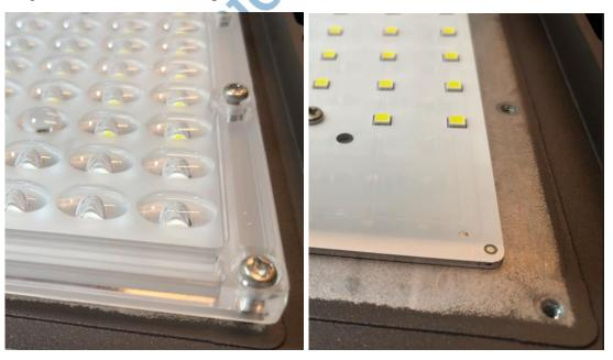
134. On information and belief, the substrate is enclosed between the heat dissipation element and said housing element; for example, the metal-core printed circuit board is enclosed between the solid-metal body and the frame and transparent window.
