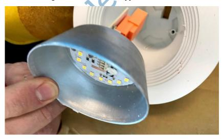
220. On information and belief, 170001-DW-US products include at least one light emitting diode (LED) thermally coupled to the heat sink; for example, 170001-DW-US products include multiple LED light sources mounted to and in thermal communication with the solid metal backing.
