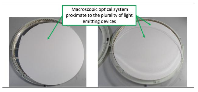
62. On information and belief, Material Number 203646A includes a microscopic optical system for diffusing the illumination created by the plurality of light emitting devices subsequent to the redirection by the macroscopic optical system, the microscopic optical system configured to retain the off-axis distribution of the illumination; thereby providing a desired level of blending of the predetermined wavelengths ranges. For example, this limitation is shown below.
