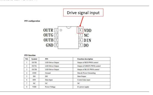
Image edited from WS2811Signal line 256 Gray level 3 channel Constant current LED Driver IC data sheet
