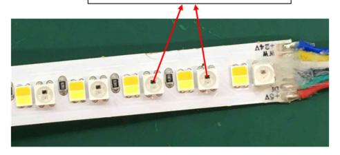
114. On information and belief, Model H6072 includes a power input electrode common to the plurality of controllers, and a power output electrode common to the plurality of light source devices. For example, this limitation is shown below.
