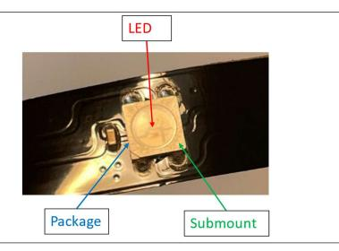
50. On information and belief, Model H6102 includes a package for the LED die including a submount, wherein the submount incorporates at least one second electronic component for controlling the LED. For example, this limitation is shown below.
