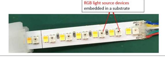
112. On information and belief, Model H6072 includes a plurality of controllers embedded in the substrate. For example, this limitation is shown below.
