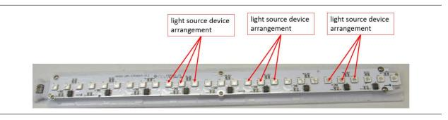
80. On information and belief, Model H6062 includes a plurality of light source device arrangements arranged in a line extending from the power connection, with adjacent light source device arrangements in the line connected together with an electrical connector arrangement comprising at least one power supply line and at least one power return line, the connector
