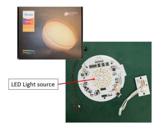
65. The testing of products shows that Model H6055 includes a LED light source including a plurality of colored LEDs operable to emit one of a plurality of spectral outputs as a function of at least one current flowing through said plurality of colored LEDs each current of the at least one current having a variable time average flow.
