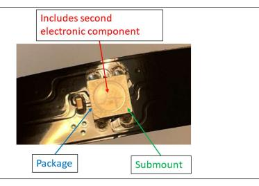
51. On information and belief, Model H6102 includes a package for the LED die including a submount, wherein the submount incorporates at least one second electronic component for controlling the LED, wherein the at least one second electronic component is coupled between the first electronic component and the LED die. For example, this limitation is shown below.
