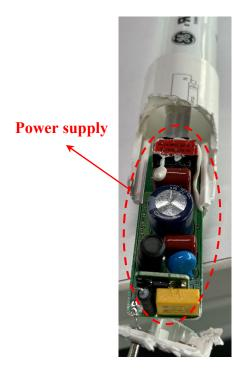
71. The power supply module comprises a rectifying circuit and a filtering circuit coupled to the rectifying circuit:
