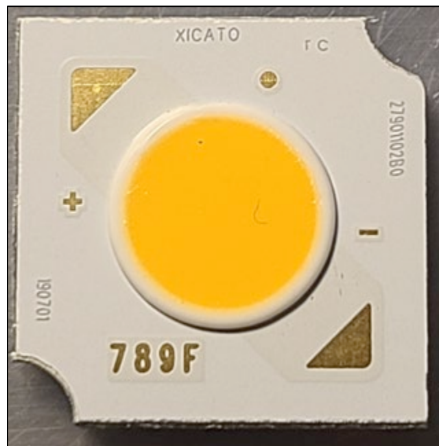
(g) The Xicato XOB06902710X3321 comprises an electrode wiring pattern on the primary surface of the substrate. The anode and cathode side patterns extend from their respective electrode lands under the resin frame and electrically connect to the LED chips.
