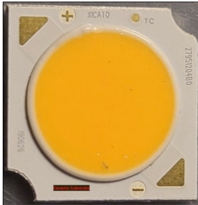
(b) The Xicato XOB09952715X3621 comprises a light emitting element disposed on the substrate by means of an adhesive resin.
